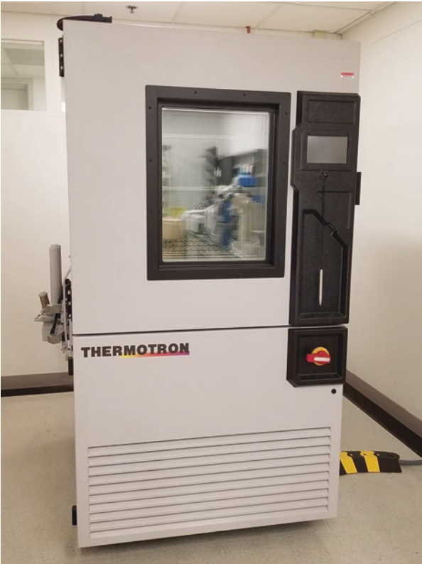
Fig. 4 Environmental chamber used for freeze-thaw measurements
