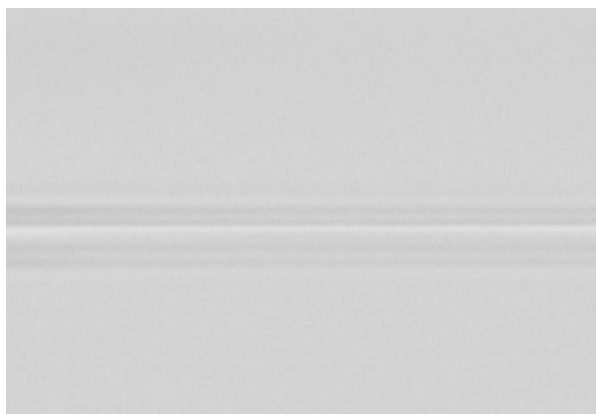
Fig. 11 Artifact from MFI subvisible particulate measurement in high concentration formulation samples when using placebo or water as blank
